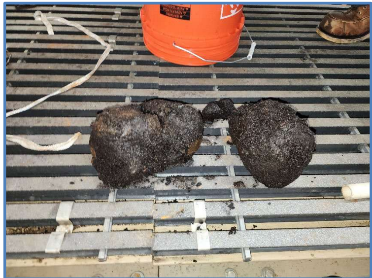
Figure 2/3: "Mudballs" from Filter 1, Cell A. Extremely large and comprised primarily of filter media bound together with manganese and iron "sludge".
