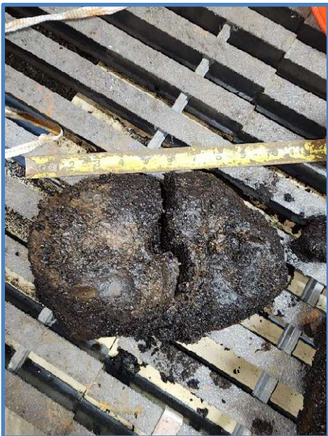
Figure 2/3: "Mudballs" from Filter 1, Cell A. Extremely large and comprised primarily of filter media bound together with manganese and iron "sludge".
